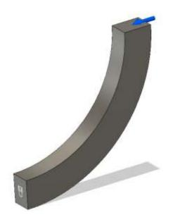
This, for simplicity is modeled as a plane stress case where the third dimension is small compared to the other two. The conservation of momentum and the generalized Hooke's law in the case where all body forces are negligible here means that,
